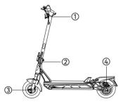
Check 1234 of the scooter before riding. Firm or not. Tighten the screws if there is any sign of loosening.
