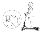
• Step 5: During riding, try to release the throttle and pull the brake lever.
