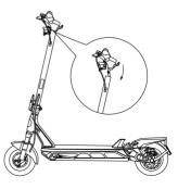
3. Tighten the screws onto three sides of the stem with the hexagon wrench.
