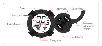
1) Speed step setting Can adjust with button.
